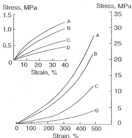
Figure 1 – Examples of Stress-Strain curves typical of elastomeric materials
